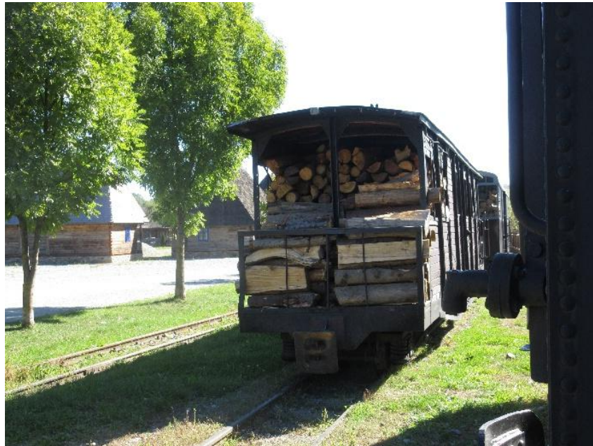
Fig.12. One of the vans used to carry wood fuel for the steam tank locomotives on the Vaser Valley railway. These are coupled immediately behind the locomotive and act as tenders to augment the limited space for timber on the engines themselves. (Photograph: David Murray-Smith).
