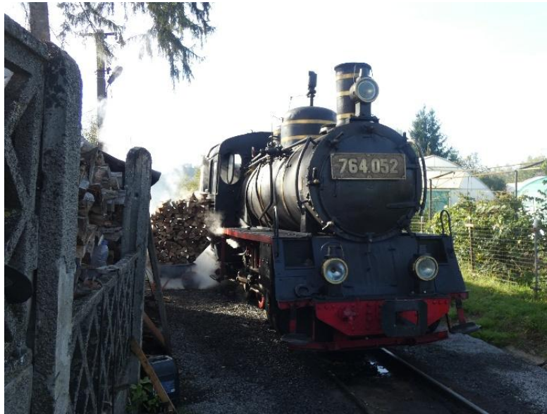
Fig. 4. Scene on the Mocănița Sovata. The 760mm gauge 0-8-0 No. 764 052 is being loaded with wood. (Photograph: David Murray-Smith).
