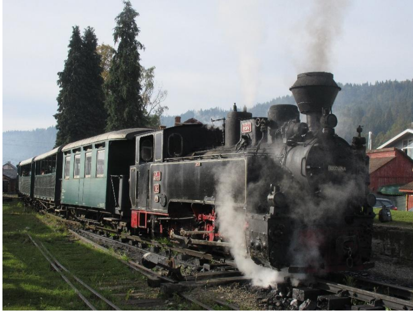
Fig. 14. Built at Reșița in 1957, 0-8-0T 764 431 stands at Gara Moldovița at the head of a train for Argel. (Photograph: David Murray-Smith).
