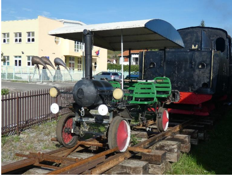
Fig. 6. An unusual steam-powered rail vehicle in store at Sovata station. The tender in the background belongs to 0-8-0 No. 764 055, also in store. (Photograph: David Murray-Smith).
