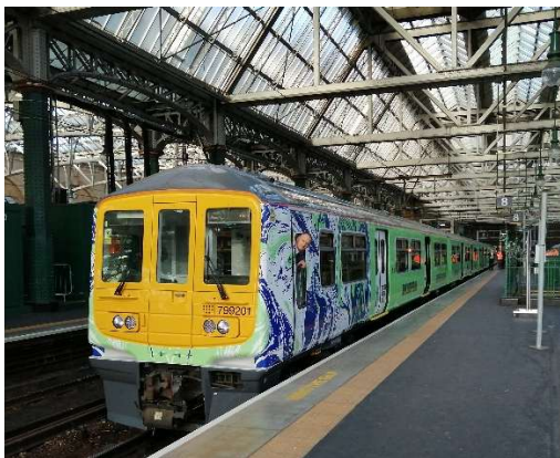
Figure 4. The Porterbrook/BCRRE Class 319 electric multiple unit which has been converted for hybrid fuel cell/battery operation. This view shows the unit at Glasgow Central Station before a demonstration run to Barrhead using electric traction only for COP26 delegates and invited guests.
