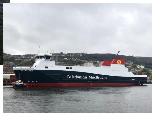
Glen Sannox, 94m x 17m, 1,000 pax, 130 cars, 34 crew, est. cost £175m, power 5,900kW, speed 16.5 knots
