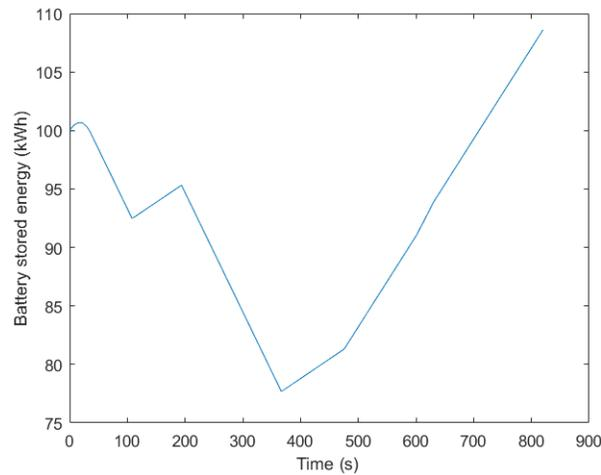
**Figure 8.** Battery stored energy time-history from inverse simulation.
