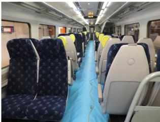
HSTs for ScotRail InterCity services are being refurbished at Wabtec's Doncaster site as these are released by GWR. New seats, sliding doors and a retention toilet are being fitted in each passenger coach. There will be seventeen 2+5 sets and nine 2+4 sets. The target is to have all ScotRail sets in service by the May 2019 timetable, though the longer trains will not be able to operate into Glasgow Queen Street until the station refurbishment giving longer platforms is completed.
